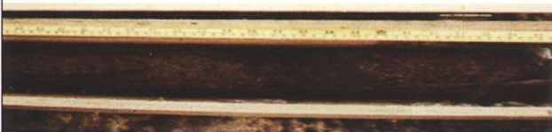
● Dense sand and stiff clay. Drilled by our surface set diamond core bit, with Coreline.
