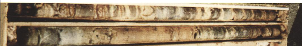
● Keuper marl, gypsum, clay cored and presented as it should be. Drilled by our Taper Tungsten core bit, with Coreline.
